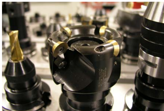
A sampling of some of the varieties of solid and insert cutting tools available.
